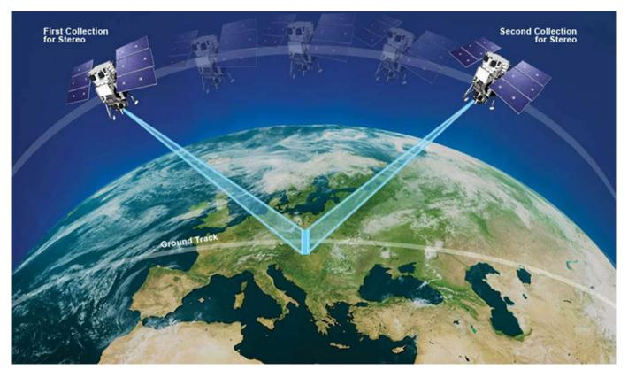
In-track stereo collection mode. The sensor collects two shots (45-90 seconds apart) of the same location by adjusting its camera. *Source: Maxar.*
